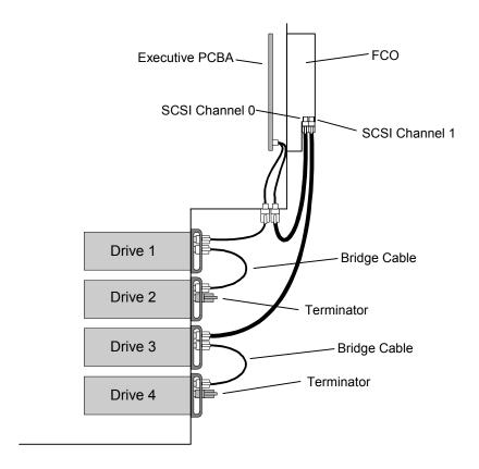
Figure 6-7 TLS-54xx, 64xx and 84xx Cabling Diagram
